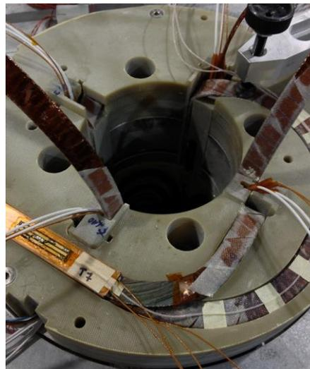
CCS sensor mounted on superconducting cable with thermalisation pad
